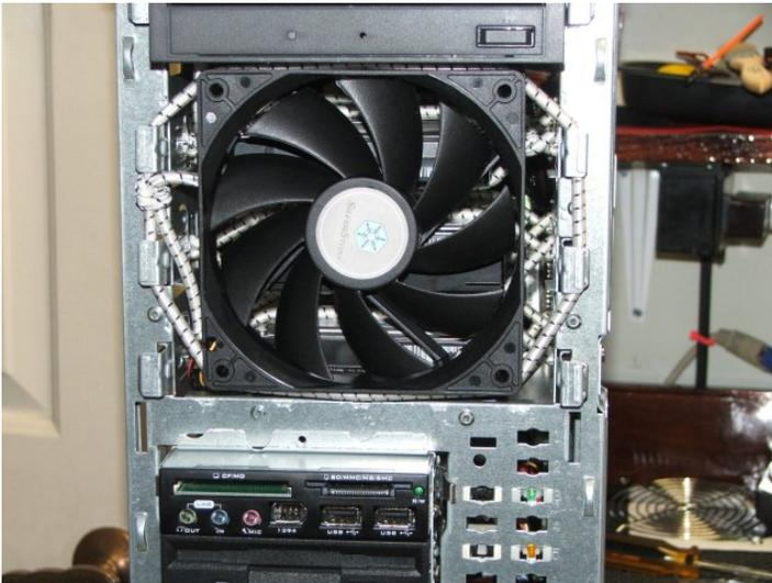
You lightly burn the nylon cover after cutting, knot it properly and it should outlast the PC for quite a few years. I then mounted a 120mm Silverstone quiet fan using the remainder of my cord, and, along with two 80mm Silverstone quiet fans in the back and the stock cpu fan for the AMD-64 3500+, the PC is virtually silent from two feet away. Note too, I used two long screws in the bottom of each drive to act as stops to keep the drives in place even if you tip the unit violently on its back.
