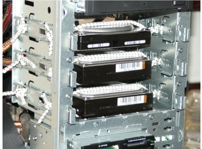
Since that time, I've built two more similar computers using the same method and even cutting two holes in the front for fans on a PC I sent my oldest son. That one moves a very large volume of air over four hard drives, video card and a very hot CPU. In spite of the amount of air flowing through the case, it's virtually silent. ♦
