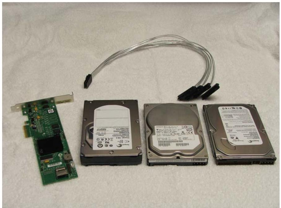
To the right of the controller card is the new 15K Seagate Cheetah, a Hitachi 80G SATA drive and a new Seagate 160G ATA (or PATA).
