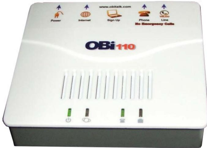
It's less than five inches on a side and 1-1/2 inches tall. On the back it has two telephone jacks, One Ethernet jack and a power supply socket for the power cube. So you cable it to your router, plug your telephone in the correct jack and power it up. You configure it – more about that in a moment – and it becomes a telephone. And you did it without even discussing it with Verizon.
