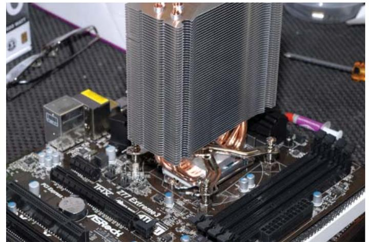
the bottom left. In the photo at the top, the CPU has been installed, and in the next photo, we see the CPU cooler installed on top of the CPU. In the photo with the cooler, on the lower right is where the memory modules will go and to the left is the slot where we will install the video card. I should note that the moth-
